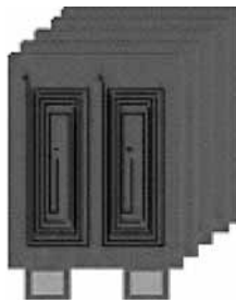
Figure 43: PRiME™ sensor multi-layers printed wiring board
