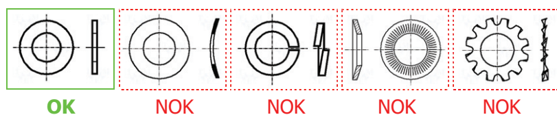
Fig. 9: Washer types allowed for direct contact with LEM transducer's brackets
